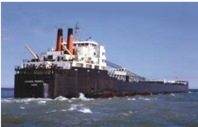
▲ Canadian Progress (1968/21,436gt) of Upper Lakes Shipping is a typical modern self-unloader, with a box-like hull and a superstructure set well aft. She was built by Port Weller Dry Docks, on the Welland Canal, to the then maximum dimensions of 222.51m by 22.94m. Photographed on 17 June 1972.
