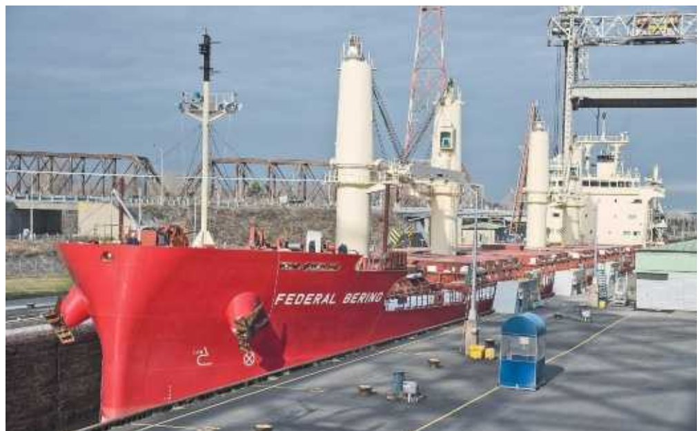
▲ The 20,789gt Federal Bering, seen transiting the Saint-Lambert Lock, is one of six similar Seaways ships built by Japan's Oshima Shipbuilding for Canada's Fednav during 2015. GILLES SAVOIE
