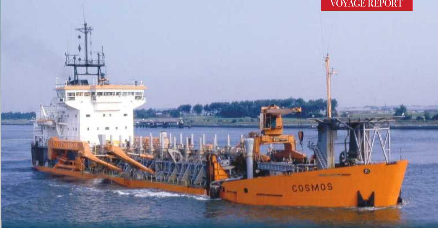
▲ The trailing suction hopper dredger Cosmos (6163g/1980) heading down the Maas with a full load of spoil.
