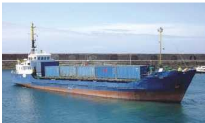
▲ The flat-bottom design of the ships used mean they are ideal for operating from tidal berths if need be.
