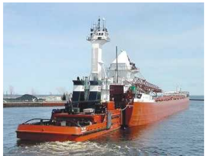
▲ A stern view of the ATB combination Victory (tug) and James L. Kubler (barge), discloses the latter's hull shape, once the 1953-built bulk carrier Reserve but cut down for barge usage in 2008. SCOTT BEST
