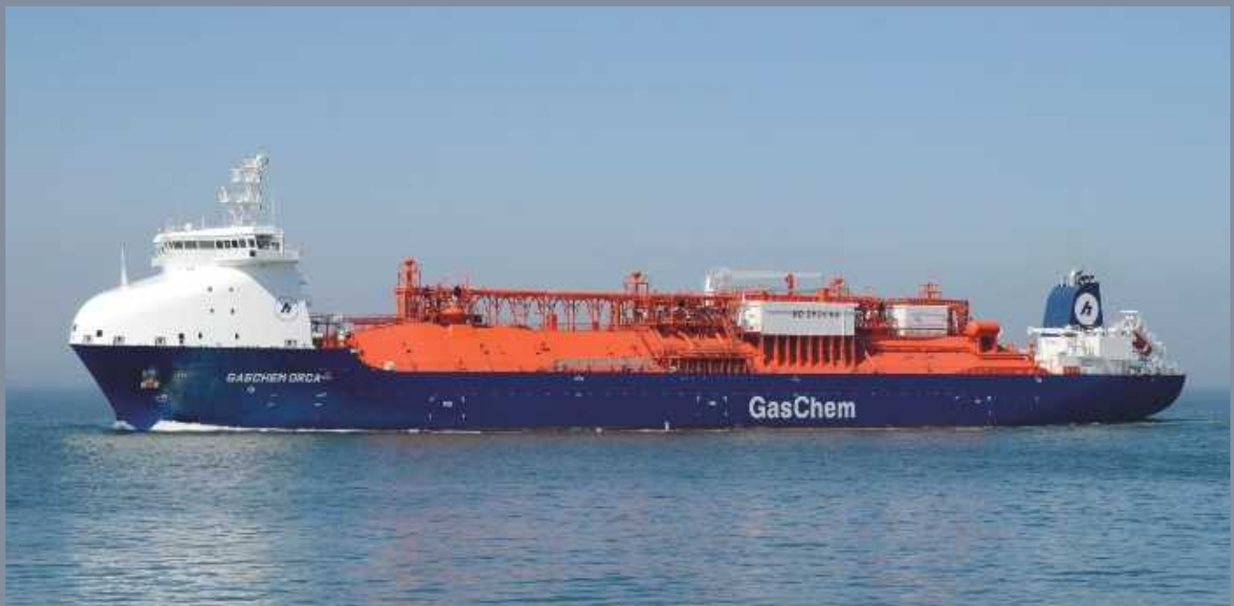
▲ Arriving at Teesport on 19 April, the Liberian-registered 21,600-ton Gaschem Orca is a new breed of LPG tanker visiting the Tees. The 188m vessel has a service speed of 16.5 knots. Owned by Hamburg-based Gaschem, she was constructed by Sinopacific Shipbuilding Group, Shanghai, China and delivered in 2017. DAVID FRASER
