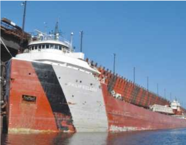
▲ Completed in 1952, and retro-fitted with a self-discharging conveyor boom in 1982, the 25,300dwt Philip R. Clarke can discharge her seven cargo holds at a rate of 6,700 tons per hour. DAVID RUFF
