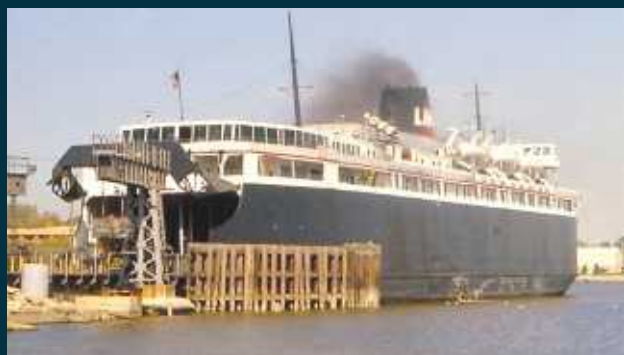
▲ A coal-burner still in operation on the Lakes is the 1952-built Badger, which is powered by two Skinner Unaflo reciprocating steam engines fed by coal-burning Foster-Wheeler boilers. JIM SHAW
