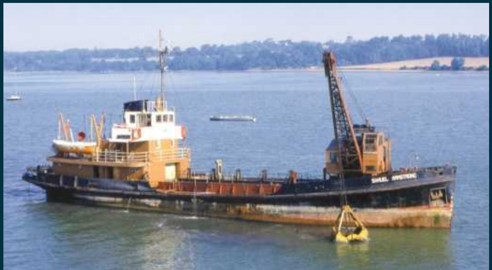
▲ The grab dredger Samuel Armstrong (364g/1956) helping keep the River Orwell channel clear.
