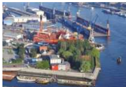
▲ Blohm and Voss shipyard from the air. Note the two floating docks, Nos.10 and 11, in the River Elbe, as well as the two smaller floating docks, 16 and 6, in front of the dry dock Helgen. Blohm and Voss have been building ships in the heart of the city of Hamburg since 1877. Today, the shipyard continues not only to build warships and commercial vessels, but also carries out numerous refits and conversions at its shipyard in Hamburg.
