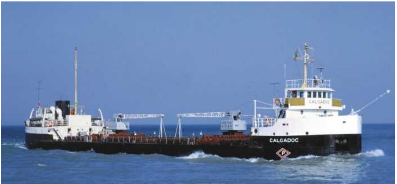
▲ Calgado (1956/2,293gt) was built at the Georgian Bay port of Collingwood for N. M. Paterson & Sons, Thunder Bay. Her Fairbanks Morse engines developed 1,280bhp. Her certificate allowed her to undertake limited coasting voyages between Belle Isle and New York. She was sold in 1975 and renamed El Salinero. On 21 September 1982 she foundered in Mexican waters. Photographed on 31 October 1971.
