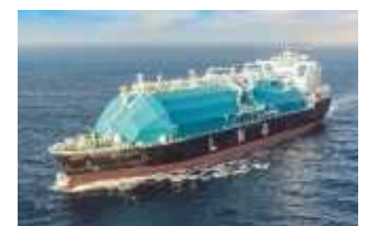
▲ The new MOSS-Type Seri C Class LNG carriers use an Integrated Hull Structure (IHS) that encloses four MOSS-Type spherical tanks. MISC
