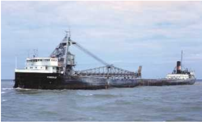
▲ The self-unloader Pinedale (1906/7,126gt) spent her first 56 years in American ownership and her last 16 in Canadian ownership as a member of the Reoch Transports fleet. The 156m ship was built by Detroit SB Co, which also supplied her 1,600ihp triple-cylinder engine. Her career ended in 1978 with demolition at Hamilton, Ontario in 1980. Photographed on 10 June 1972.
