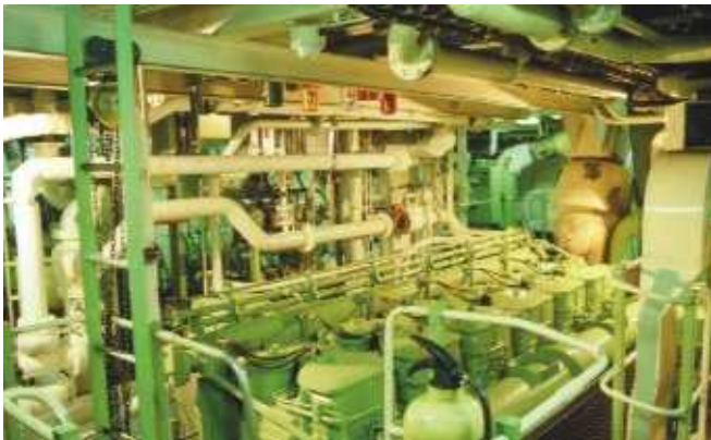
▲ Shell Marketer's K Major six-cylinder Mirrless diesel.
