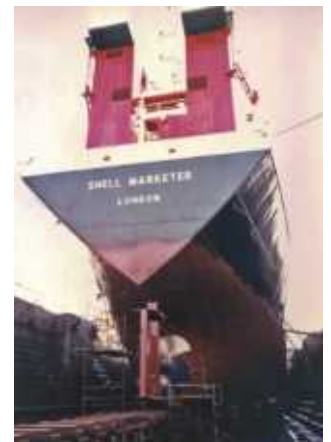
▲ Shell Marketer in dry dock at Sunderland in October 1984; her controllable pitch propeller and high lift rudder are clearly visible.
