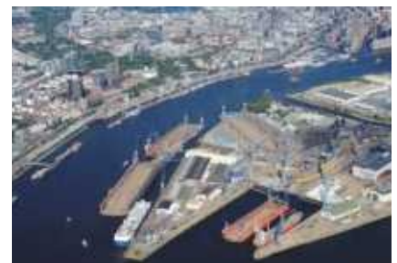
▲ Blohm and Voss shipyard from the air. Note the two floating docks, Nos.10 and 11, in the River Elbe, as well as the two smaller floating docks, 16 and 6, in front of the dry dock Helgen. Blohm and Voss have been building ships in the heart of the city of Hamburg since 1877. Today, the shipyard continues not only to build warships and commercial vessels, but also carries out numerous refits and conversions at its shipyard in Hamburg.
